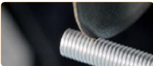
Burr-free cutting of thread rods
